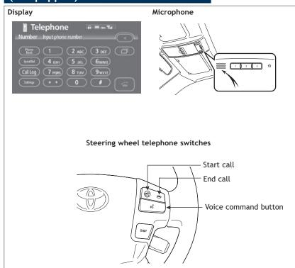
Bluetooth® technology allows dialing or receipt of calls without taking hands from the steering wheel or using a cable to connect the telephone and the system.
